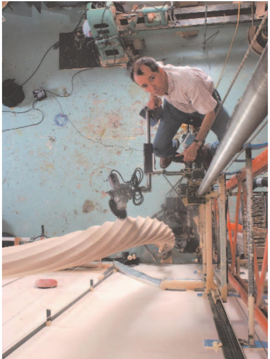
Perched on a tractor seat that travels up the column, Macnab manipulates a 5½" sawblade mounted in a slow-speed buffer to control the cutting of the flutes.
